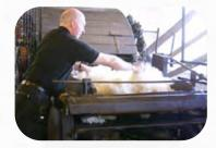
The process of carding gets all the knots out of the wool and straightens it ready for spinning.
