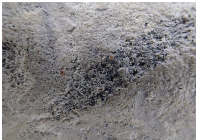
Fig.5 (top left) tomb of Bishop John Morgan, craved from Beer Stone. Fig. 6 (bottom left) close up of Beer Stone chalk texture. Fig 7 (top right) Characteristic burrow structures in Beer Stone. Fig. 8 (bottom right) close up of dark glauconite grains in burrow.
